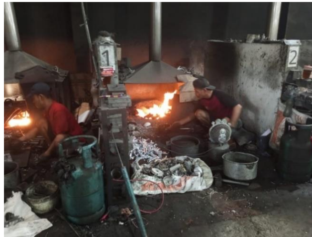
Fig. 1. The Metal Melting Process with a Gas-fired Furnace
