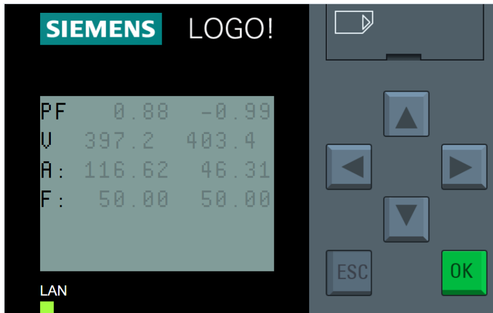
Fig 11. Schneider Multimeter Data shown in Block Module's Display.
